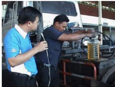
3. Prepare to measure time and write the test form. Start the engine and time, and take records. Time may be 15, 20, or 30 minutes depending on the fuel volume consumption. Fuel consumption should be about 700 ml.
