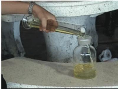
2. Place the fuel for test glass bottle near the truck's fuel tank, then remove the intake and the return fuel tubes from the truck's tank to the test bottle. Be careful that air shouldn't go in-line.
